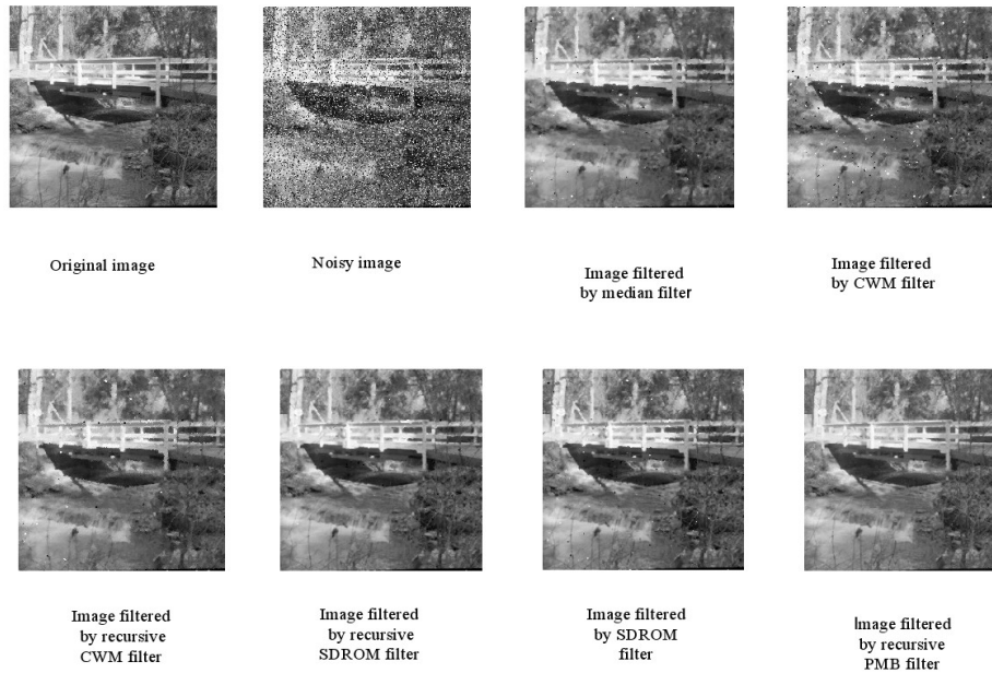
Figure 5. - Comparison of the restoration performance of different filtering type for the Bridge image corrupted by 20% fixed-valued impulses
