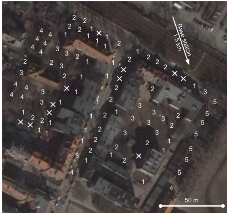
Fig. 2. WiMAX coverage hole effect – measured coverage of WiMAX base station in 3.5 GHz band. Stable modulation profile chosen by client terminal: white X - no communication, “1” – BPSK, “2” – QPSK, “3” – QAM16, “4” – QAM64 1/2, “5” – QAM64 3/4).
